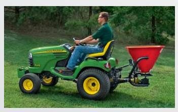
**Rear Spreader**Fertilise in a single pass with the rear-mounted spreader.
