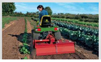
**Power Tiller**Prepare seedbeds or control weeds will minimum effort. Mounts easily to rear 3-point hitch. Tractor PTO delivers torque for fast, deep tilling.
