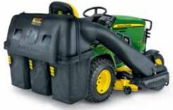
The 500 litre 3-bag collection system is also available and fits the X740, X748 and X749 mowing tractors.
